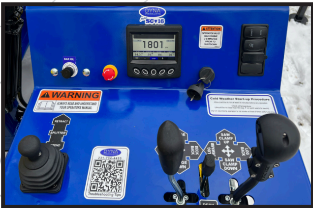
WEATHERPROOF SMART ENGINE CONTROL PANEL READS AUTO-CYCLE SPLITTER (SC-16 RAPID SPLIT)
