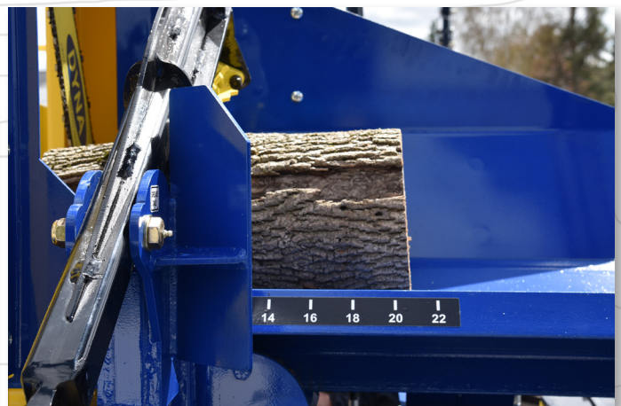
MEASURES LOG REMAINING ON TROUGH
