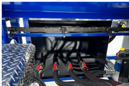
IMPROVED HOSE ROUTING REDUCES DEBRIS BUILDUP
