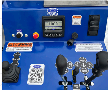
WEATHERPROOF SMART ENGINE CONTROL PANEL READS AUTO-CYCLE SPLITTER
