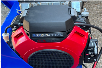
20 HP ELECTRIC START HONDA ENGINE
